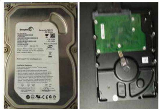
Figure 1.5: Two sided view of a sealed hard disk unit
